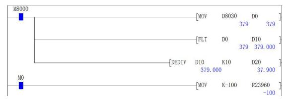
In the above figure, when M0 is closed, the value -100 is transmitted to the
