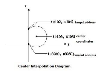
Note 1: The current address of X and Y must be on the same circle as the destination address.
