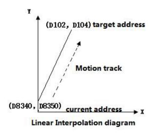
In the Center interpolation: D100 is speed, D102 is the X-axis target address, D104 is the Y-axis target address, and D106 is the center X address. D108 is the center Y address. Y0 and Y1 respectively pulse the X-axis and Y-
