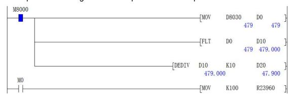
If the current temperature is 37.9°C, the actual test is 47.9 ° C, the error is 10 ° C, you need to modify the size correction register, show as below:
